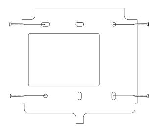
If installing BioStation A2 on a concrete wall, drill holes, insert PVC anchors, and fix them with fixing screws.
