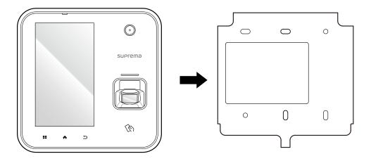
Connect BioStation A2 to the bracket by rotating the product fixing screw of BioStation A2.
